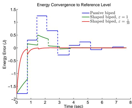
Fig. 5: Convergence has more desirable behavior with energy shaping. Smaller values of  $\varepsilon$  offer better convergence.
