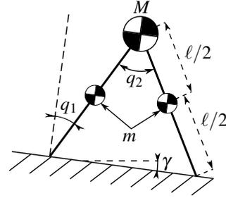
Fig. 1: Compass-gait biped with walking down a slope.
