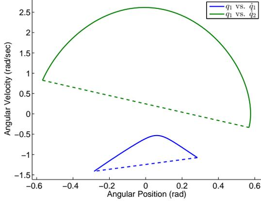
Fig. 2: Limit cycle of the passive compass gait biped.
