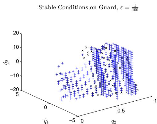
Fig. 6: The domain of attraction restricted to the guard for both the shaped (blue '+') and passive systems (black 'x').
