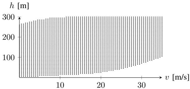
Fig. 4: The domain of the controller enforcing (10) on the system (4), i.e.  $\llbracket \psi \rrbracket$ . Each point represents a discrete state. 90% of the points in the  $h$ -coordinate have been removed for visibility.
