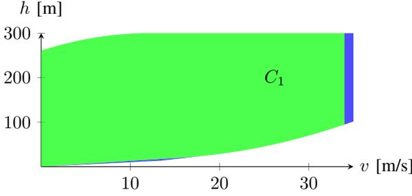
Fig. 3: The overlapping sets  $C_1 \subset C_2 \subset C_3$ . The control-invariant set  $C_1$  is pictured in green and is entirely visible.  $C_2$  and  $C_3$ , which are both subsets of  $G$ , are colored in blue and constitute the region from where  $C_1$  is reachable.
